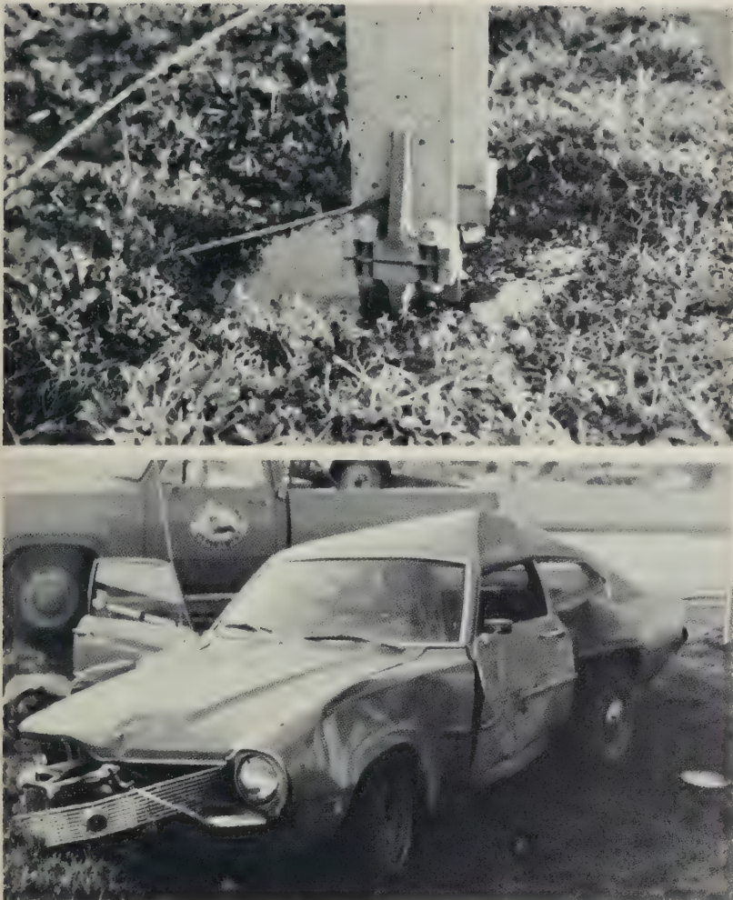
Figure 1.— This base for a breakaway sign satisfies present requirements for conventional-sized automobiles, but when struck "side on" by a compact automobile severe damage resulted.
