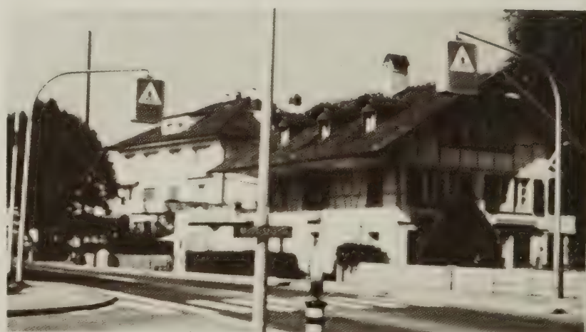
Figure 3.—Internally illuminated pedestrian signs frame a marked crosswalk in Bern, Switzerland.
