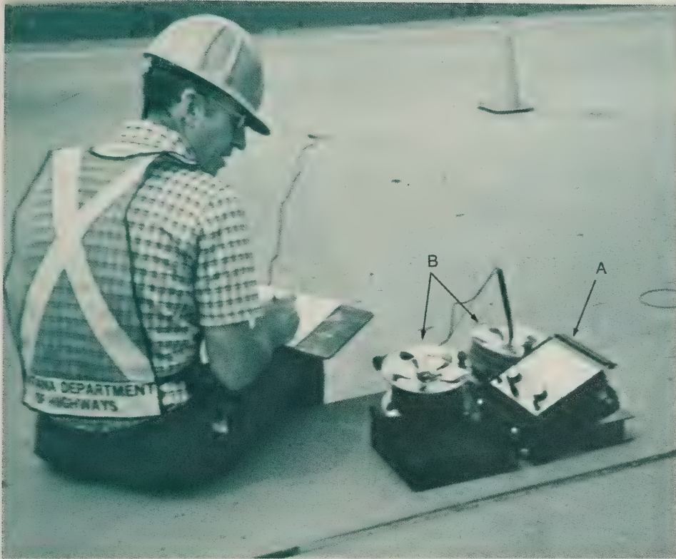
Figure 3.—Electrical corrosion detection device consisting of a very high impedance voltmeter (A), coils of lead wire (B), and a half cell (C); locates corroding rebar.
