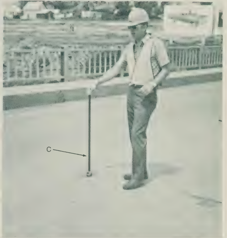
Figure 3.—Electrical corrosion detection device consisting of a very high impedance voltmeter (A), coils of lead wire (B), and a half cell (C); locates corroding rebar.
