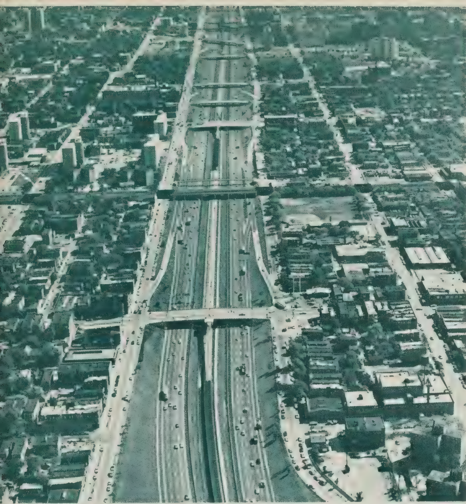
Figure 14.—An application of a heavy traffic corridor featuring a series of signalized diamond interchanges with mass transit in the median, all within a narrow right-of-way.
