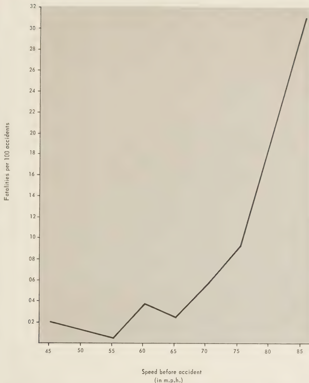
Figure 6.—Average reported fatalities per 100 single-vehicle accidents observed in rural areas by selected speed before the accident.
