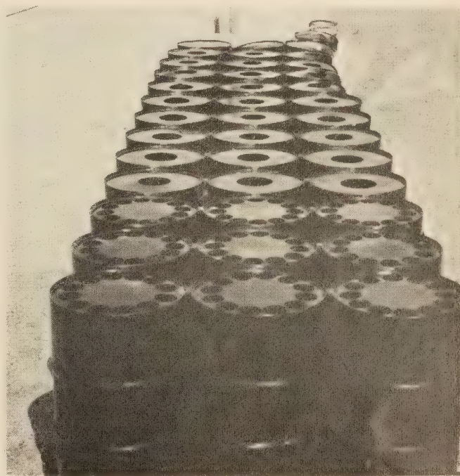
Figure 25.—A 57-m.p.h., 20° test with a 4,200-lb. vehicle of a barrier designed for median bridge piers.
