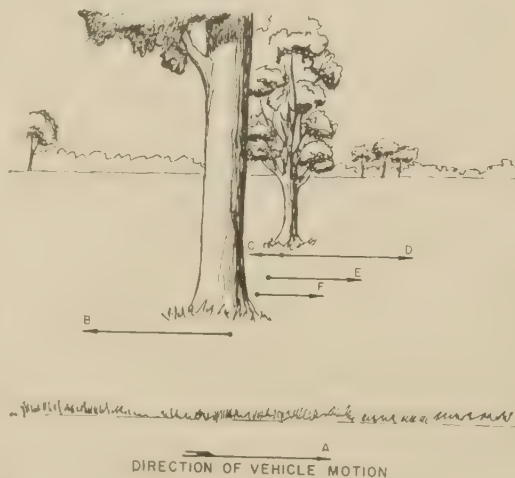
Figure 14.—Motion parallax curl. Illusion shown at right angles to vehicle's line of movement. Vehicle moving in direction A, inducing vectors B in foreground tree and vectors C in background tree. If foreground tree is fixated, background moves to right with velocity D. Ground positions between trees have linearly decreasing velocity vectors that produce appearance of rotation.
