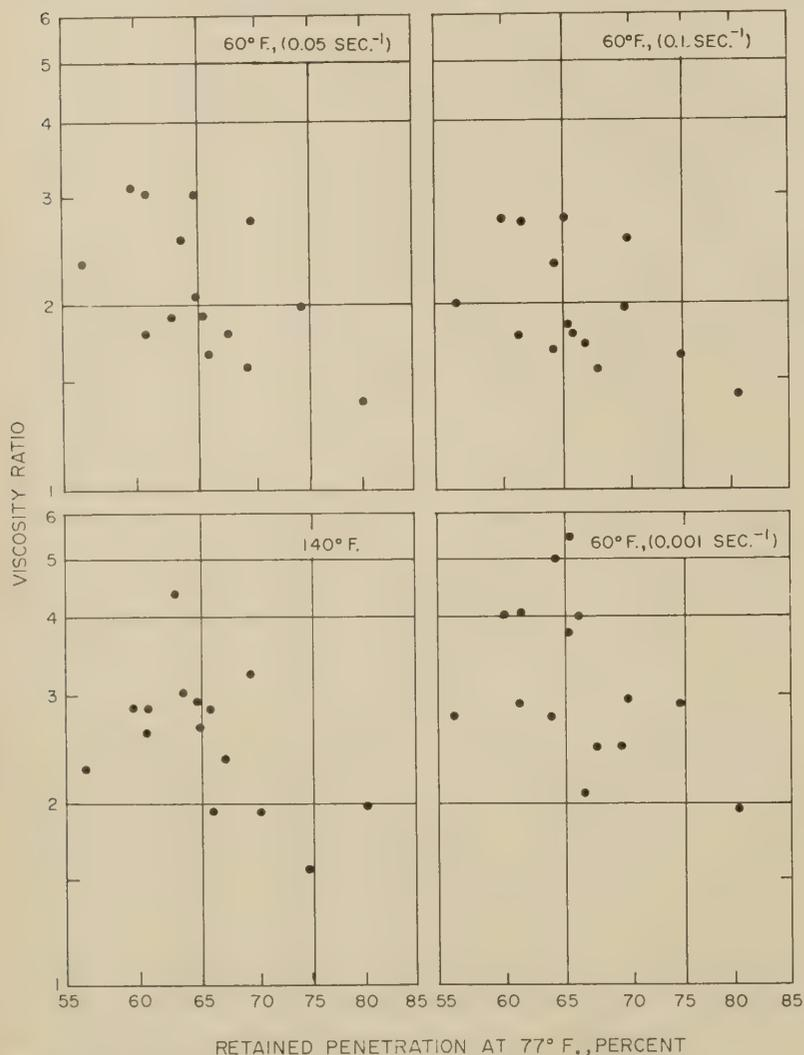
Figure 12.—Relation of percent retained penetration at 77° F. and viscosity ratios at 140° F. and 60° F. for AC-20 viscosity grade asphalt cement.
