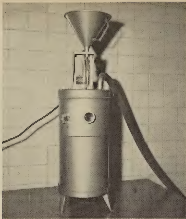
Figure 20.—Abrasiometer, door closed during test, and hopper at top.
