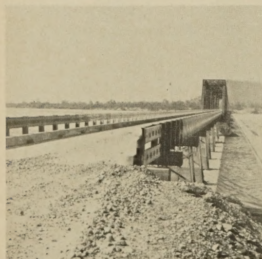
Figure 9.—Test mounting boards for exposure A near end of right guardrail at east abutment of Mile 27 Bridge.
