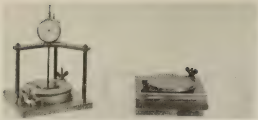
Figure 15.—Georgia volume change test: one specimen soaking, one specimen drying.
