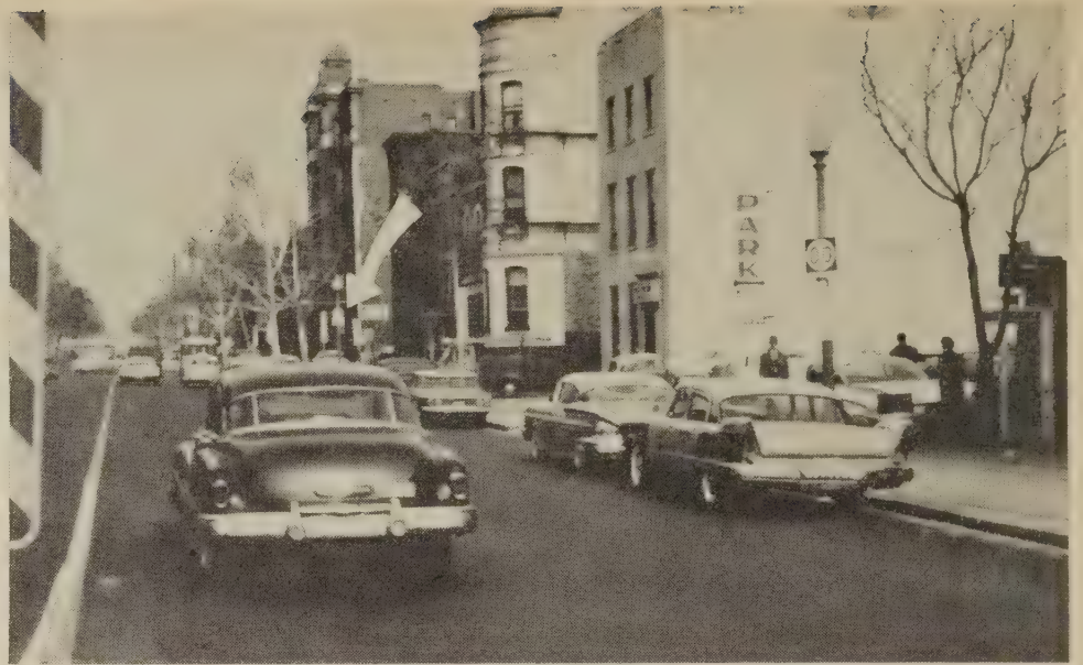
Figure 6.—Illustration of how well the white route marker on a black square shows up against both dark and light backgrounds.
