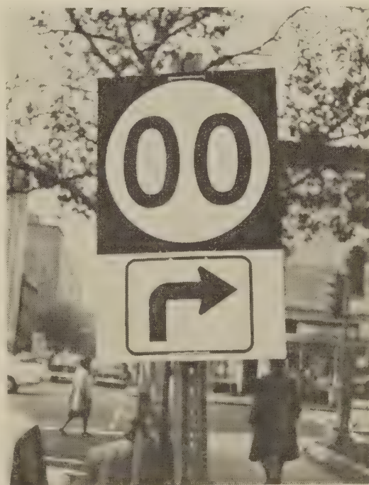
Figure 2.—Advance-turn marker assembly used for the study.
