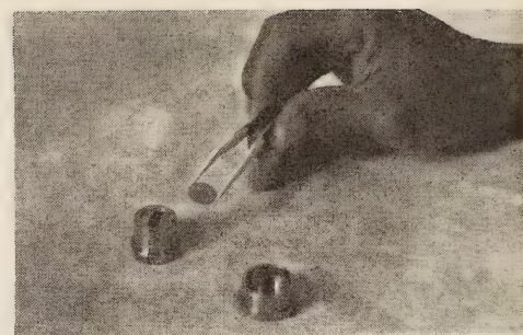
Figure 7.—Potassium bromide disk and disk holder.
