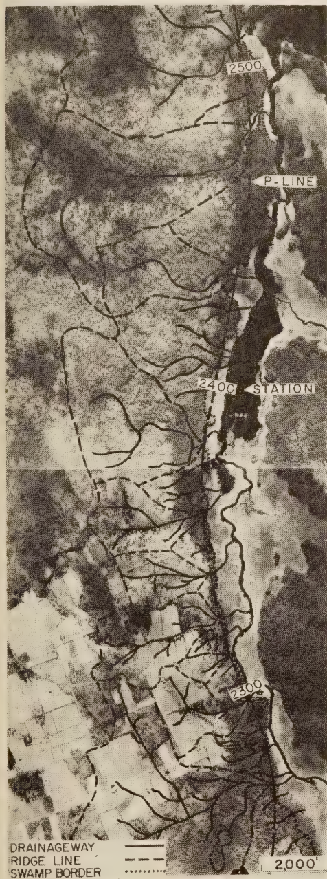
Figure 7.—Uncontrolled mosaic of drainage delineations (courtesy of the Maine State Highway Commission); watershed areas were obtained directly from the photographs.
