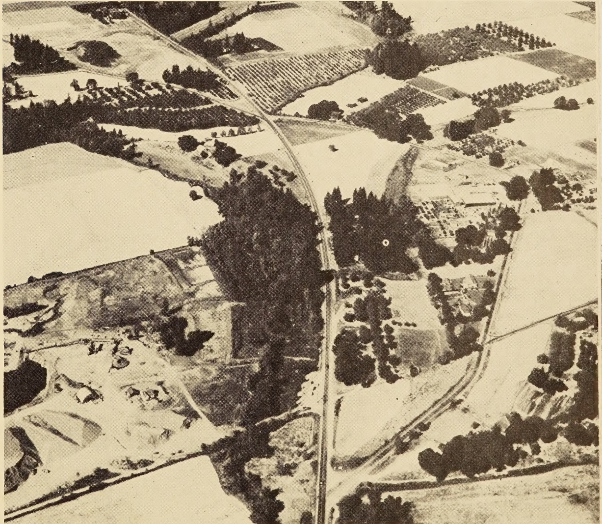
A Federal-aid secondary highway improvement in Marion County, Oreg. A sharply curved dog-leg (seen to the right) was eliminated by the new roadway.
