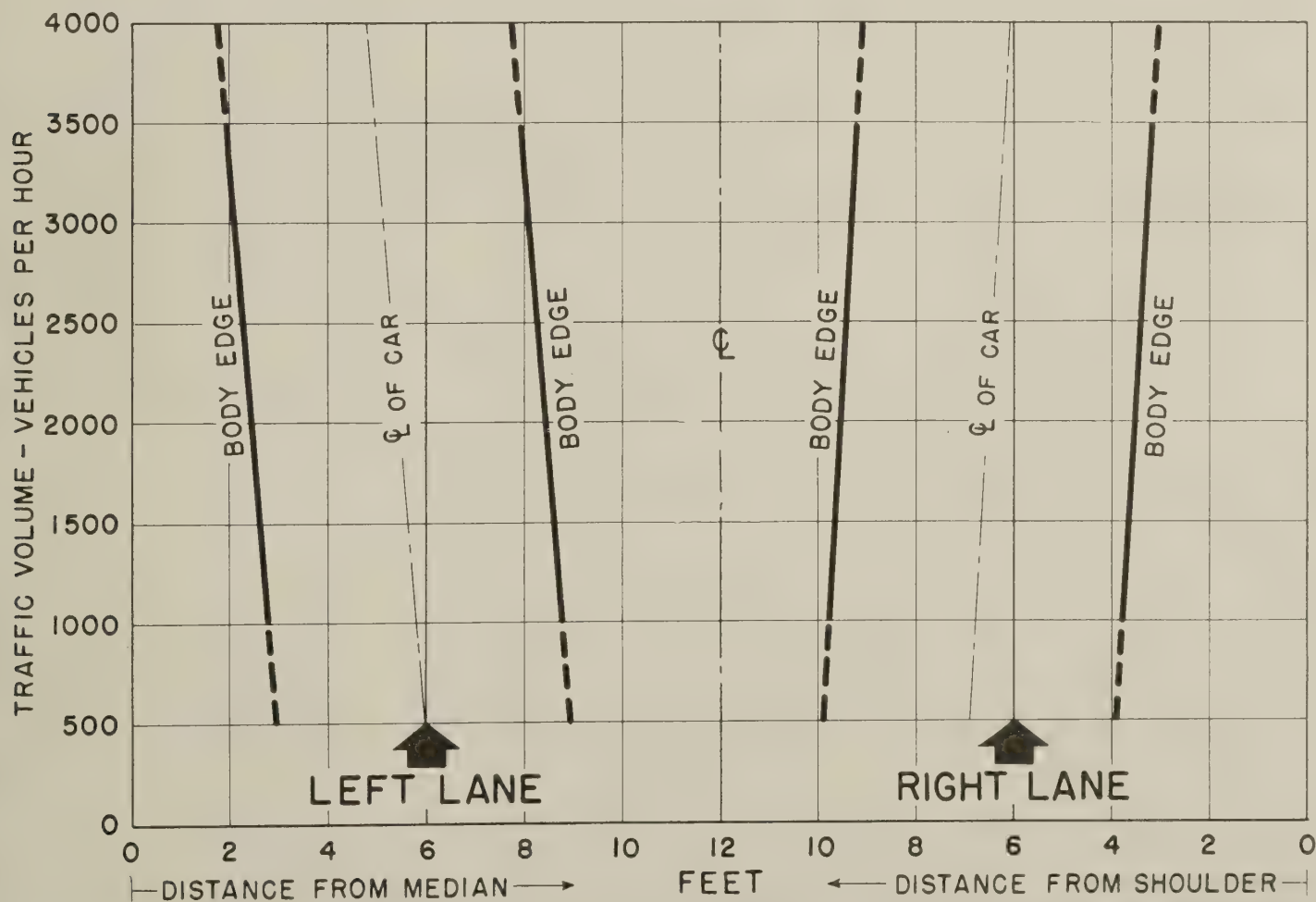
Figure 12.—Average position of passenger cars traveling in one direction on a four-lane divided highway during different traffic volumes.
