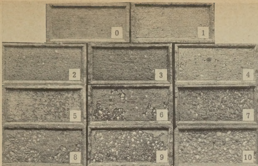
Figure 1.—Rating scale (0-10) of resistance of concrete to scaling after laboratory freezing and thawing with calcium chloride.
