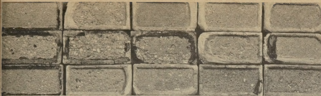
Figure 5.—Effect of single coat of mineral oil on resistance of non-air-entrained concrete to scaling after 40 cycles of laboratory freezing and thawing with calcium chloride.
