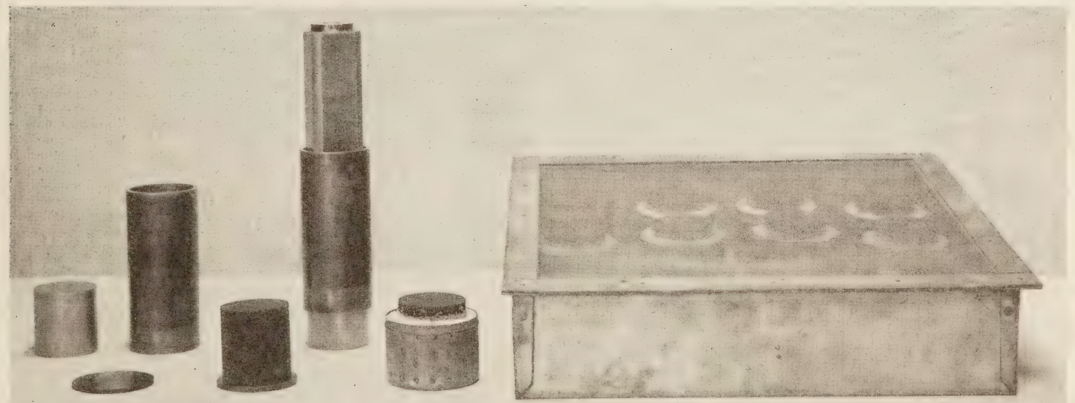
Figure 17.—Base plunger, base plate, centering and retaining sleeve, molded specimen, assembled mold, specimen supported by sand, and pan with screen cover used in oven weathering.
