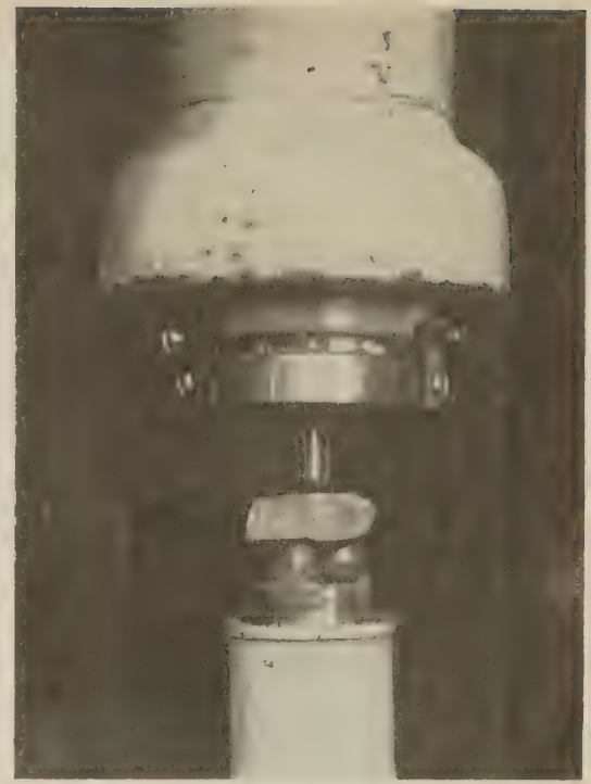
Figure 5.—Compression test for soft pieces, using a three-point support and a single-point load-bearing contact.
