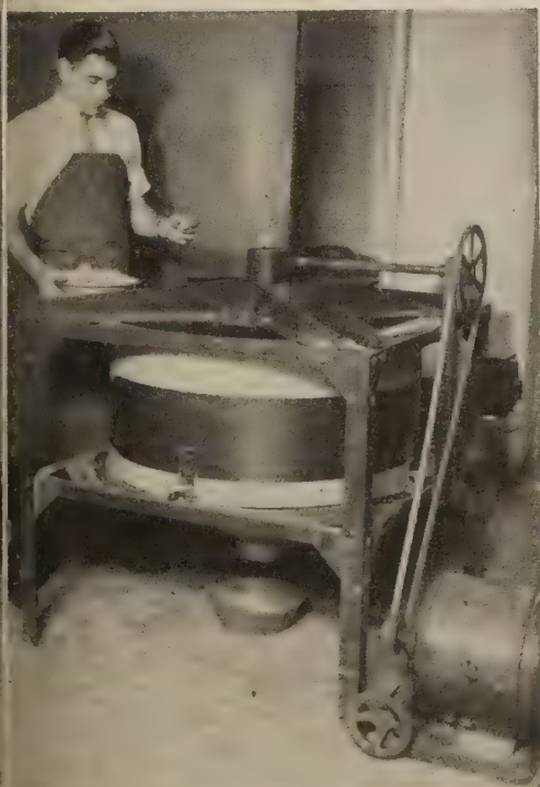
Figure 2.—The rotary soft-stone machine.
