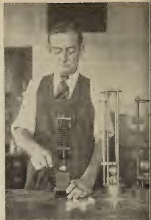
Figure 4.—Douglass stone meter in use. To the right are the toughness machines with the 1 1/8-inch and 2 1/2-inch balls.
