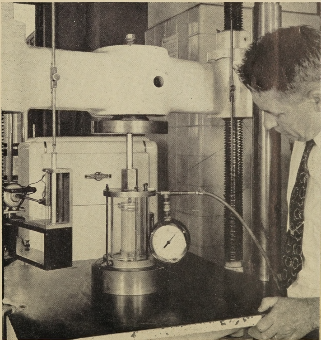
The triaxial compression test apparatus
