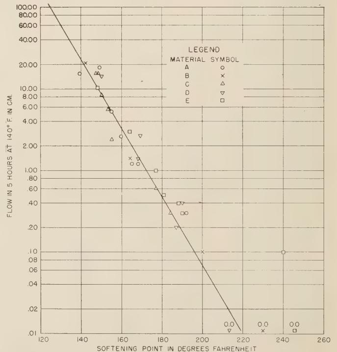
FIGURE 6.—RELATION BETWEEN SOFTENING POINT AND FLOW.
