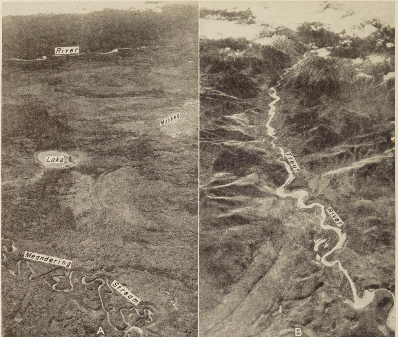
FIGURE 5.—DIFFICULT TOPOGRAPHY—(A) MUSKEG ON LEVEL GROUND, AND (B) A NARROW, TORTUOUS RIVER VALLEY.
