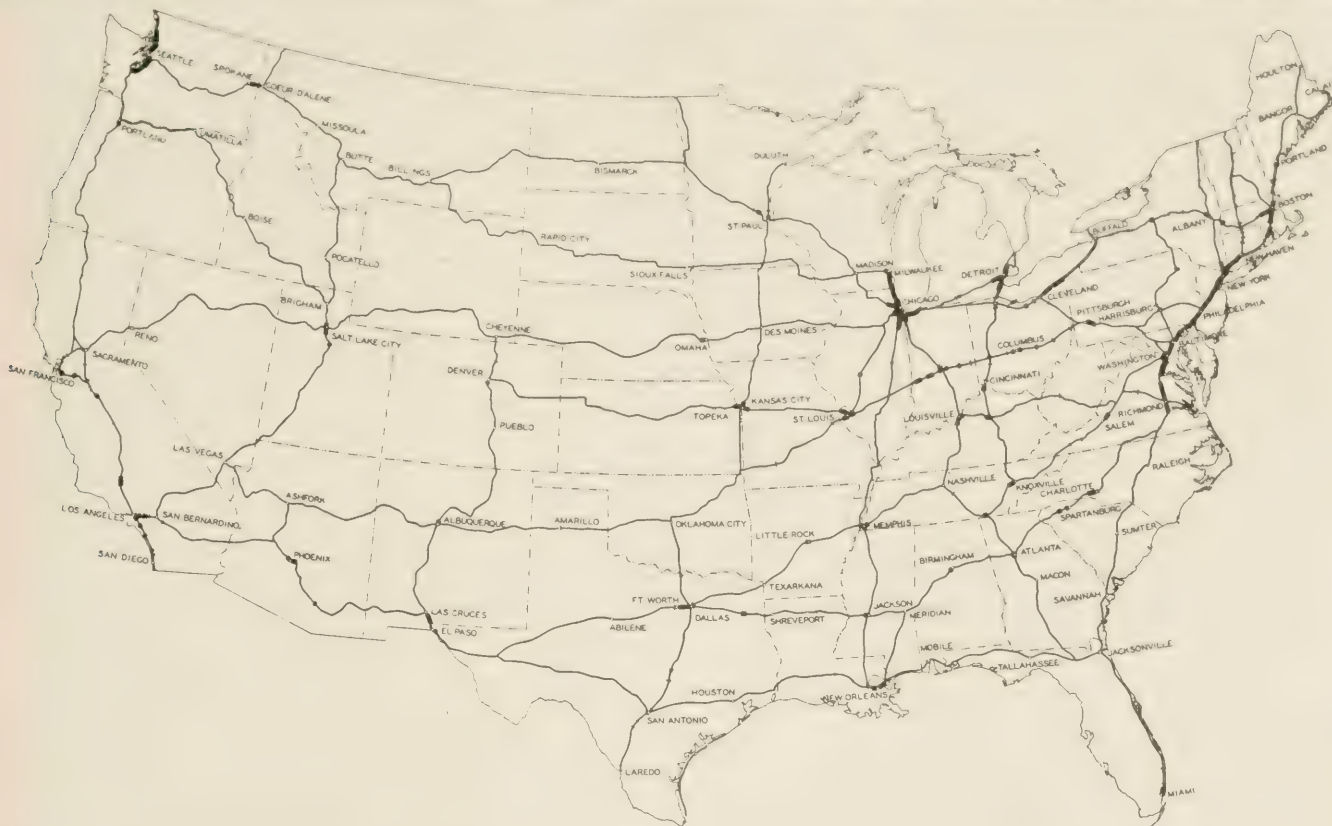
FIGURE 9.—LOCATION OF SECTIONS OF THE TENTATIVELY SELECTED INTERREGIONAL HIGHWAY SYSTEM HAVING FOUR OR MORE LANES.
