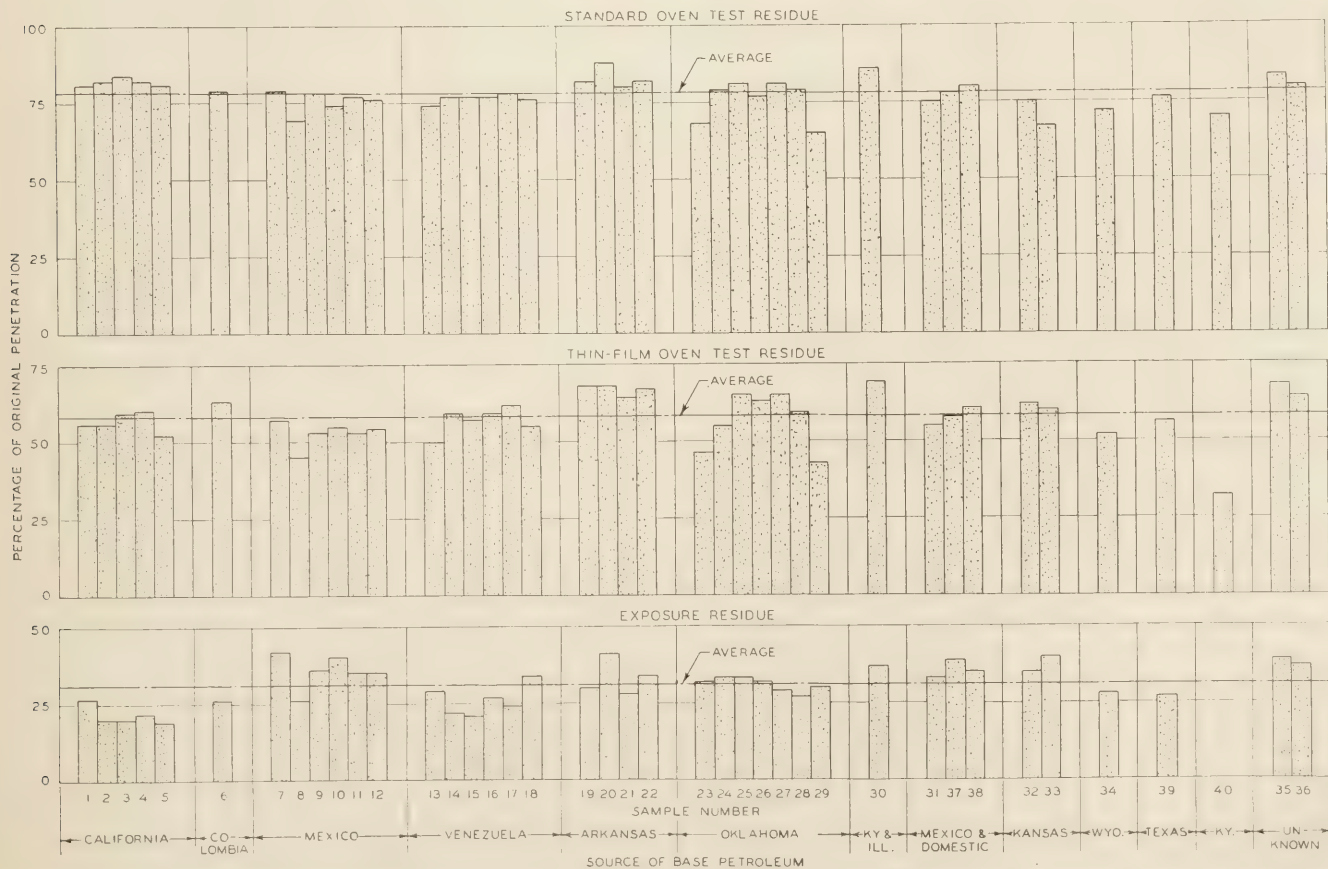
FIGURE 4.—SOURCE OF THE BASE PETROLEUM IN RELATION TO THE EFFECT OF OVEN HEAT AND EXPOSURE TESTS ON THE PENETRATION OF THE 85-100 PENETRATION ASPHALTS.
