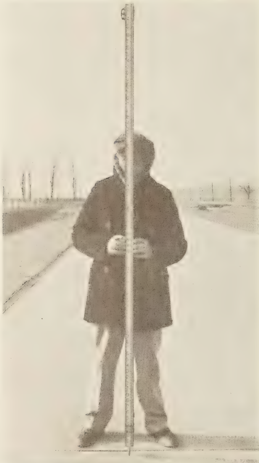
FIGURE 19.—LEVELING ROD WITH SPECIAL ATTACHMENT.
