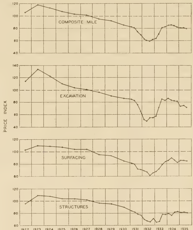
FIGURE 1.—PRICE TREND IN HIGHWAY CONSTRUCTION. AVERAGES FOR 1925 TO 1929 TAKEN AS A BASE.
