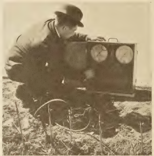
FIGURE 29.—MEASURING THE PRESSURE BETWEEN THE PAVEMENT SLAB AND THE SUBGRADE.
