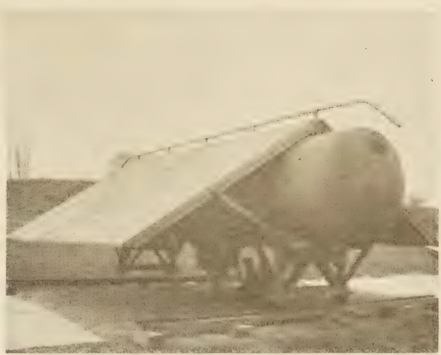
FIGURE 11.—LOADING EQUIPMENT IN PLACE OVER ONE OF THE TEST SECTIONS. THE SLAB IS COVERED WITH STRAW AND SHADED TO PREVENT WARPING.
