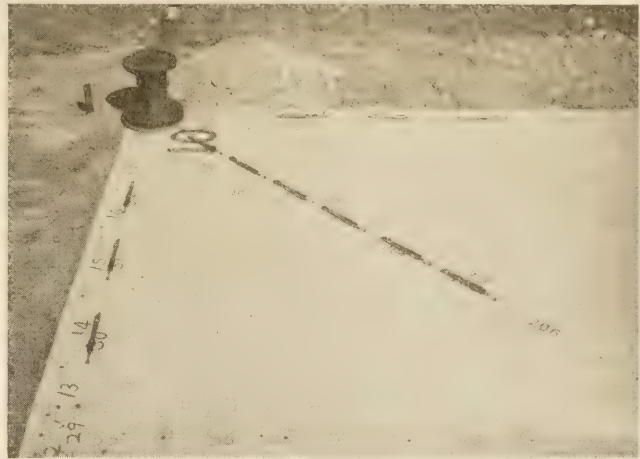
FIGURE 15.—ARRANGEMENT OF STRAIN GAGES FOR A LOAD TEST AT THE CORNER OF A SLAB OF UNIFORM THICKNESS.
