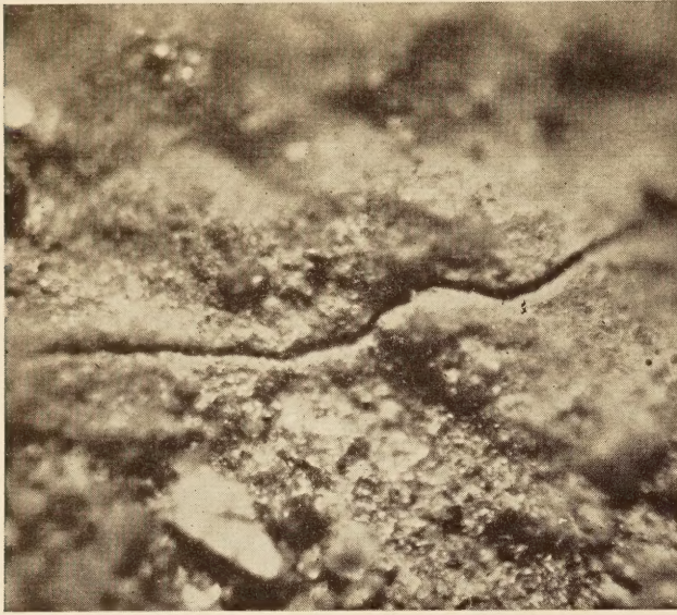
FIGURE 2.—DEPOSITS OF CHEMICAL AT EDGES OF FISSURE IN MORTAR. LENGTH OF FISSURE SHOWN ABOUT ONE-SIXTEENTH INCH. MAGNIFIED 55 DIAMETERS.
