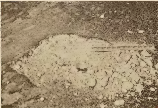
C.—CONCRETE POWDERED AND COHESIONLESS. AGE 10 YEARS
