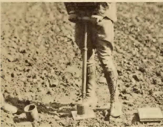
FIGURE 9.—COMPACTING SOIL IN PROCTOR CYLINDER AND DETERMINING CONSISTENCY OF FILL WITH PLASTICITY NEEDLE.
