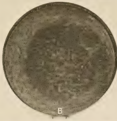
Major portion of the surface is dull, black, and pitted. Surface has shrunk and cracked. Material in bottom of larger cracks is soft and sticky. Remaining surface is very hard.
