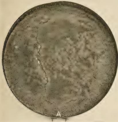
Major portion of the surface is dull, black, and pitted. Surface has shrunk and cracked. Material in bottom of large crack is soft and sticky. Remaining surface is very hard.
