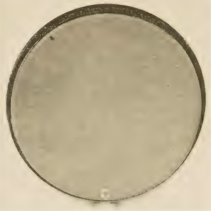
Surface is smooth and glossy to the naked eye but has a mottled appearance when seen under a glass. There is an indication of checking.
