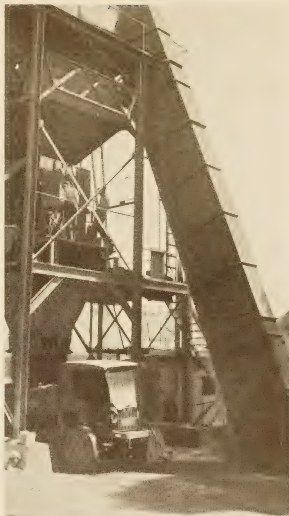
A MODERN PLANT WITH HOUSED ELEVATOR FOR HOT MATERIALS. A LARGE TRUCK IS LOADING FROM THE STORAGE BOX.
