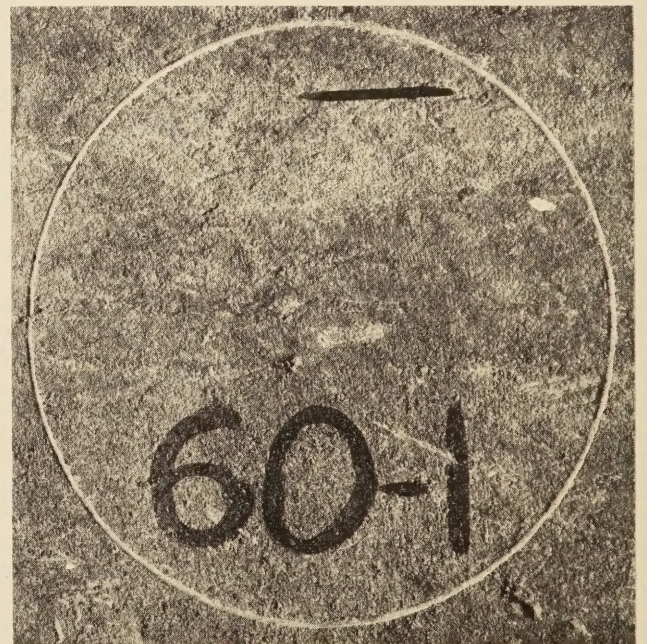
FIGURE 2.—GROOVE WORN IN SURFACE AFTER 600 REVOLUTIONS OF HARDNESS TESTING MACHINE; CIRCLE 21 INCHES IN DIAMETER.
