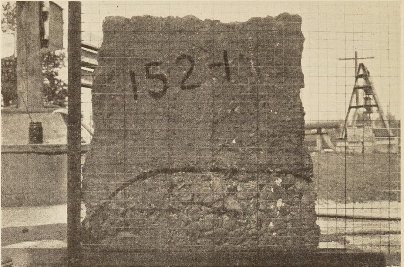
FIGURE 1.—ILLUSTRATING USE OF GRID WITH 1-INCH SQUARE OPENINGS FOR MEASURING HONEYCOMB.
