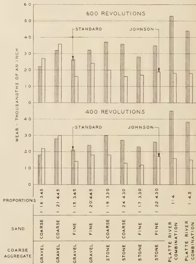
FIGURE 26.—SERIES B, EFFECT OF JOHNSON METHOD OF FINISHING ON SURFACE WEAR.
