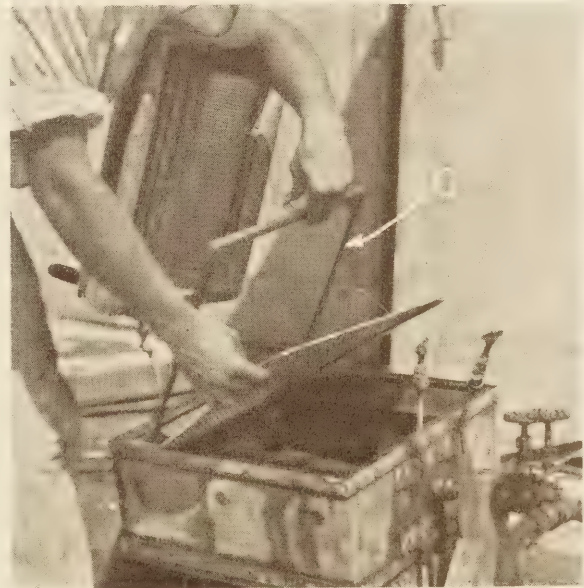
FIGURE 2.—FRAME C IS PLACED OVER THIS NO. 4 SIEVE. THIS FRAME COMES IN CONTACT WITH THE TOP COVER AND HOLDS THE SIEVE FIRMLY IN PLACE. THE TOP COVER IS THEN CLAMPED IN POSITION AND THE WATER TURNED ON
