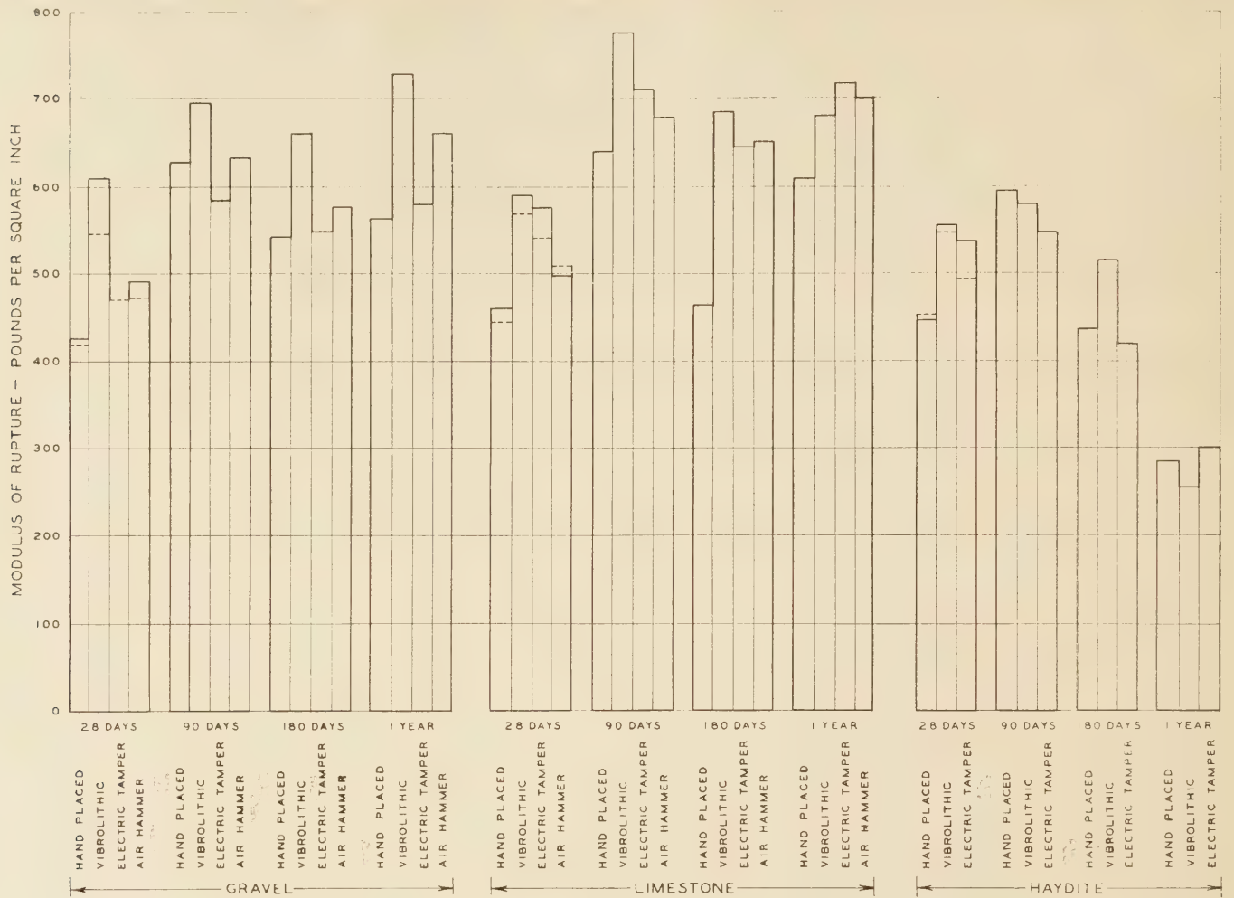
FIGURE 6.—EFFECTS OF AGE, METHOD OF PLACING, AND TYPE OF AGGREGATE ON FLEXURAL STRENGTH OF CONCRETE. VALUES SHOWN ARE MEAN VALUES OF MODULUS OF RUPTURE FOR SAWED BEAMS FROM TWO SLABS OF EACH TYPE AS GIVEN IN TABLE 4. DASH LINES INDICATE MEAN VALUES FOR LARGE SLABS BROKEN AT 22 DAYS
