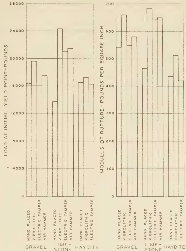
FIGURE 21.—COMPARISON OF VALUES OF MODULUS OF RUPTURE OF PLAIN CONCRETE BEAMS AND VALUES OF LOAD ON REINFORCED CONCRETE SLABS AT INITIAL YIELD POINT. IN LEFT-HAND PANEL ARE GIVEN VALUES OF LOAD ON REINFORCED SLABS AT CHANGE IN SLOPE OF LOAD-STRESS CURVES, CORRECTED TO 8-INCH THICKNESS. VALUES OF MODULUS OF RUPTURE OF SAWED BEAMS AT 180 DAYS, GIVEN IN RIGHT-HAND PANEL, ARE MEANS OF 4 TESTS ON GRAVEL CONCRETE, AND 8 TESTS ON LIMESTONE AND HAYDITE CONCRETE
