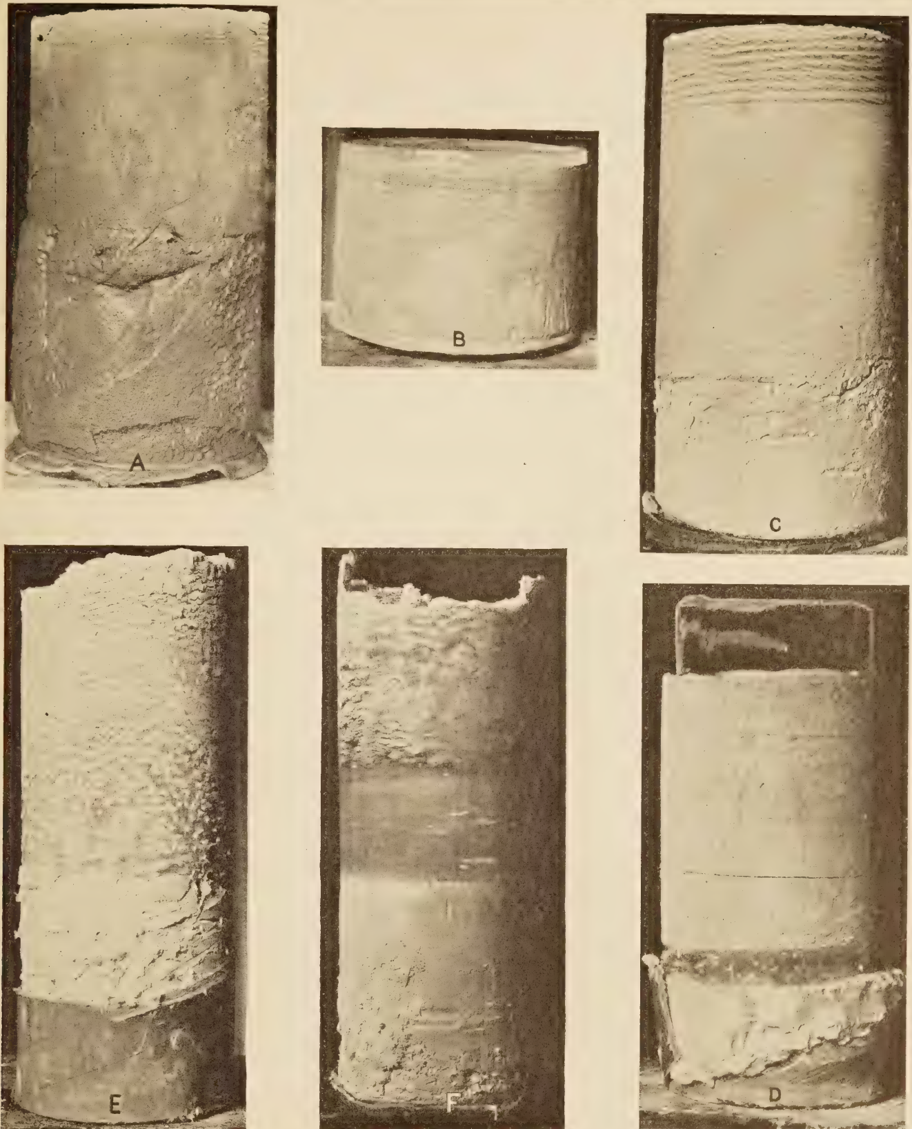
FIGURE 9.—SPECIMENS SHOWING INFLUENCE OF SOIL TEXTURE ON FORMATION OF SEGREGATED ICE: A—QUARTZ FLOUR, MAXIMUM PARTICLE SIZE ABOUT 0.07 MILLIMETER, SHOWING SLIGHT BANDING NEAR TOP DUE TO ICE SEGREGATION. B—QUARTZ FLOUR, PARTICLE SIZE 6 TO 10 MICRONS. SLIGHT BANDING DUE TO ICE SEGREGATION. C—BARIUM SULPHATE, PARTICLE SIZE ABOUT 2 MICRONS, SHOWING SEGREGATION OF ICE. D—BARIUM SULPHATE WITH ICE LAYER AT LOWER LIMIT OF FREEZING; THIN ICE LAYERS ABOVE. IRON WEIGHT ON TOP. E—LITHOPONE, PARTICLE SIZE ONE-HALF MICRON, SHOWING SEGREGATED ICE. F—KADOX, PARTICLE SIZE ONE-FOURTH MICRON, WITH LAYER OF PURE ICE 5 CENTIMETERS IN THICKNESS.
