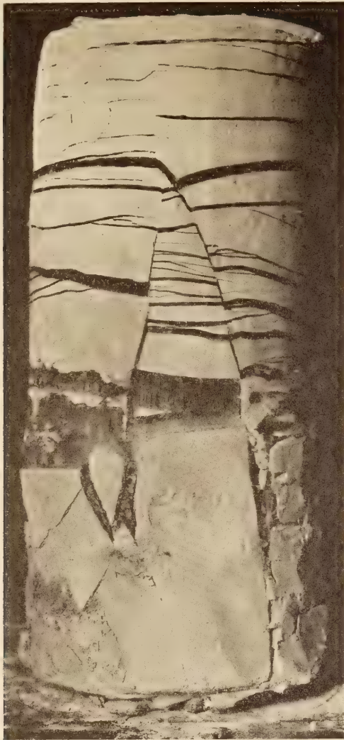
FIGURE 19.—CLAY CYLINDER FROZEN UNDER A LOAD OF 3.52 KILOGRAMS PER SQUARE CENTIMETER WHILE STANDING IN WET SAND
