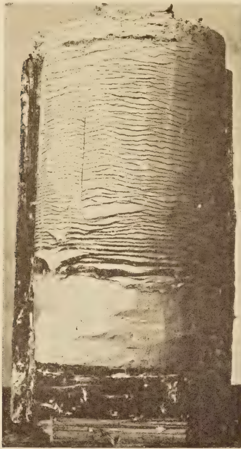
FIGURE 23.—CLAY FROZEN UNDER PRESSURE OF 15 KILOGRAMS PER SQUARE CENTIMETER IN THE APPARATUS SHOWN IN FIGURE 22
