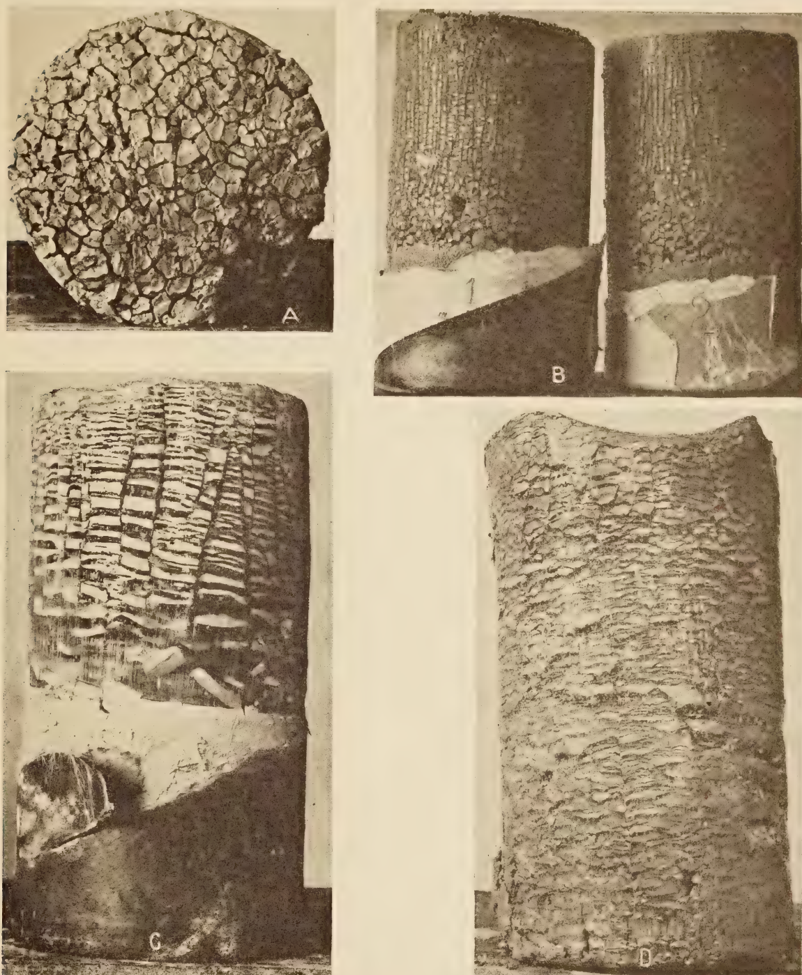
FIGURE 12.—RESULTS OF FREEZING TESTS MADE ON SPECIMENS CONTAINING BENTONITE. A.—POLYGONAL PATTERN FORMED ON FREEZING A MIXTURE CONTAINING 25 PER CENT BENTONITE AND 75 PER CENT CLAY. B.—CELLULAR STRUCTURE FORMED ON FREEZING A MIXTURE OF BENTONITE AND WATER. CARTON NO. 1 STOOD IN WATER. CARTON NO. 2 WAS SEALED AT THE BOTTOM. C.—CELLULAR STRUCTURE FORMED ON FREEZING 94 PER CENT CLAY AND 6 PER CENT BENTONITE MIXED WITH WATER. D.—THE RESULT OF FREEZING 4 PER CENT BENTONITE MIXED WITH 96 PER CENT CLAY WHILE STANDING IN WET SAND
