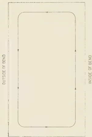
FIGURE 4.—NORMAL CONDITION OF SPIRAL FLOW IN BEND OF RIVER OR IN CLOSED CHANNEL BEND IN WHICH THE FRICTION IS GREATEST AT THE BOTTOM OF THE CHANNEL APPROACHING THE BEND
