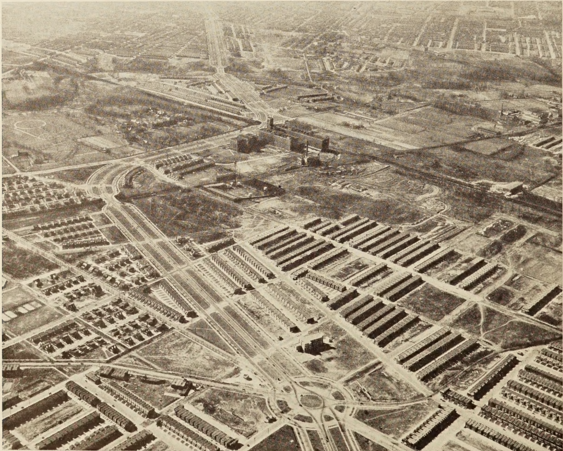
AIRPLANE VIEW OF ROOSEVELT BOULEVARD, PHILADELPHIA, SHOWING FREQUENT STREET INTERSECTIONS AT GRADE
