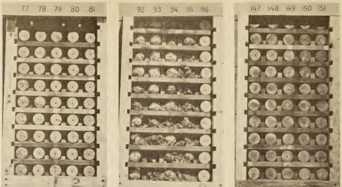
Cylinders cured in steam at 212° F. after three and one-half years in lake
