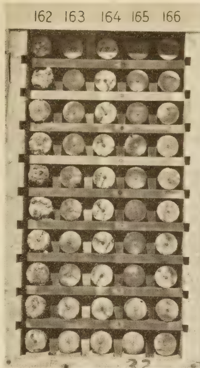
Cylinders with 4 per cent and 8 per cent admixtures of calcium chloride, variously cured
