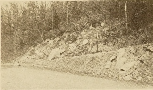
FIG. 8.—CHARACTER OF MATERIAL WHICH COMPOSES LANDSLIDE DETRITUS. NOTE ABUNDANCE AND COARSENESS OF SANDSTONE FRAGMENTS
