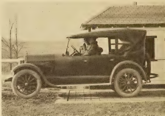
SHOWING THE SCALES USED FOR MEASURING THE DOWNWARD KICK OF AUTOMOBILES AND TRUCKS. FOR NORMAL STARTS THE AVERAGE DOWNWARD KICK OF THE 4-CYLINDER, 5-PASSENGER TOURING CAR SHOWN WAS 7.6 PER CENT OF THE LOAD ON THE REAR AXLE
