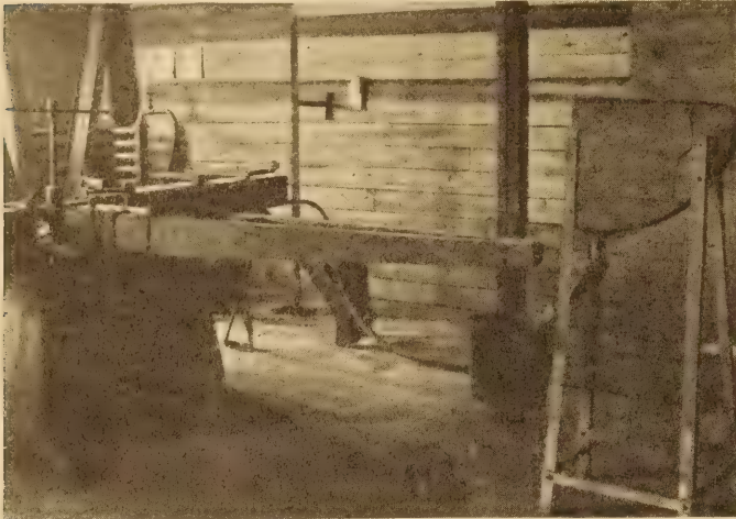
FIG. 2.—Apparatus used in determining transverse breaking strength of concrete beams
