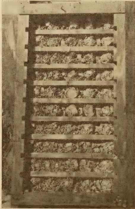
FIG. 2.—Cylinders from series 82 to 86, cured in water vapor at 155° F.
