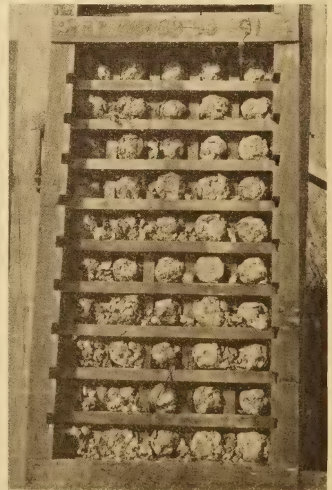
FIG. 3.—Cylinders from series 87 to 91, cured in water vapor at 100° F.
