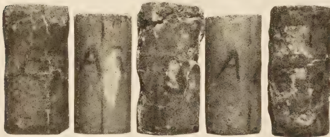
The increase in volume caused by immersion in magnesium sulphate solution is here plainly illustrated. The three swollen cylinders have been immersed in a 1 per cent solution for 38 weeks. The other two from the same lot have been kept in distilled water for the same length of time. All cylinders are 1:3 mix, normal consistency, standard Ottawa sand
