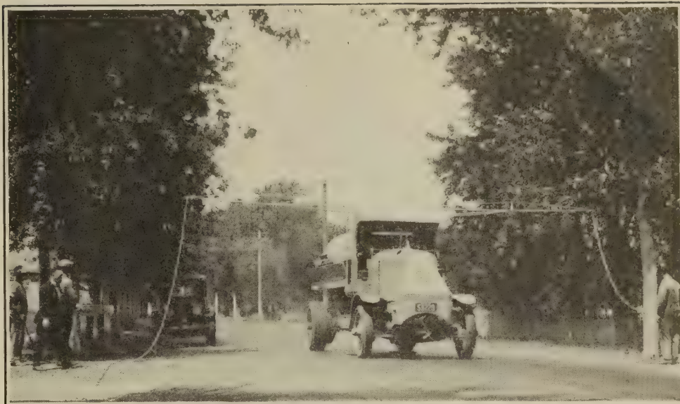
AN ARMY TRUCK CONVERTED TO SPRAY WHITWASH ON POLES IN NEW JERSEY.
