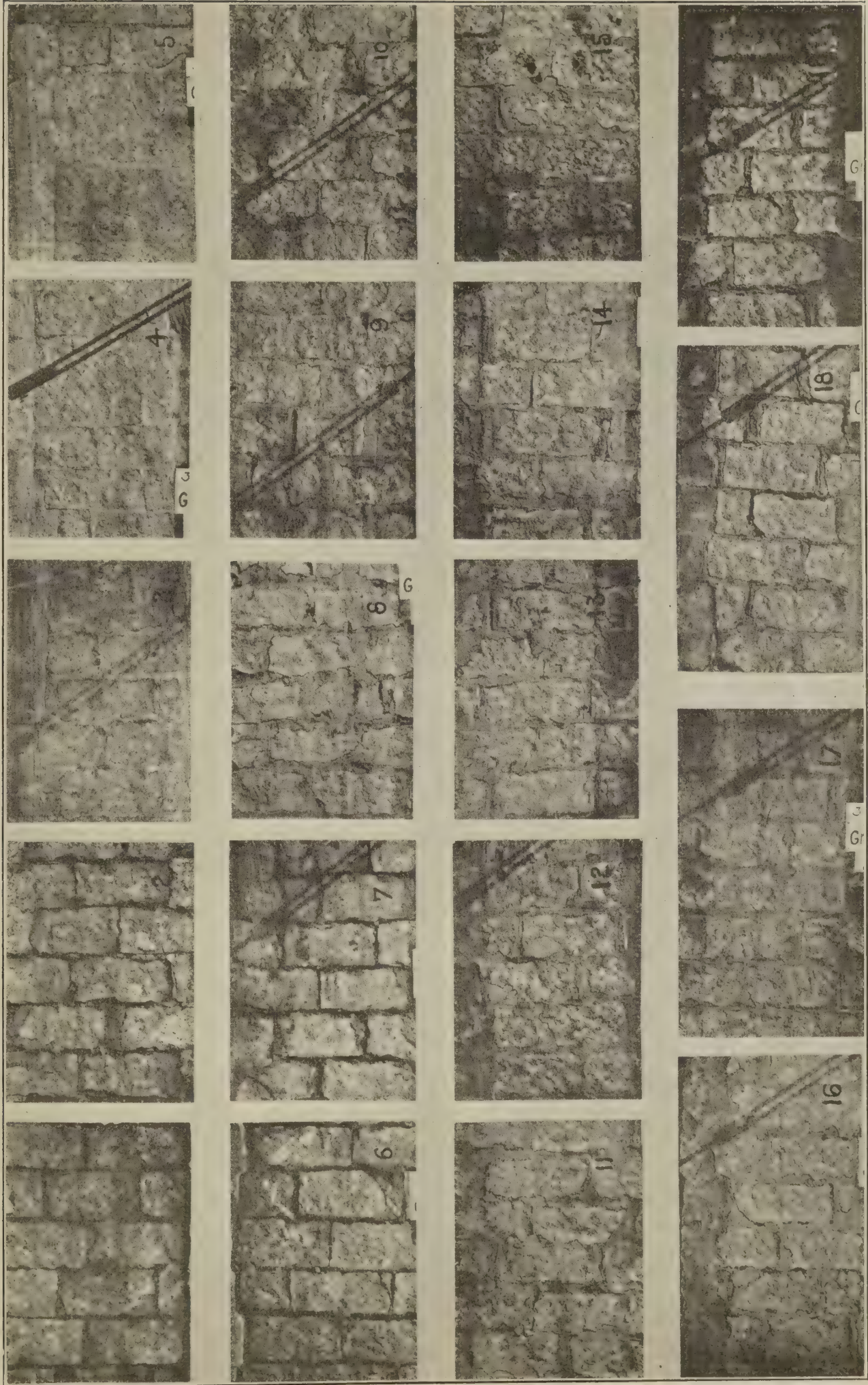
PLATE 2.—WEAR TESTS OF GRANITE BLOCK—6,000 RUNS
