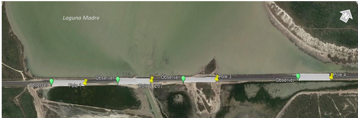
Figure 128. Annotated Aerial Photograph of the Original SH 48 Resight Survey Stations along the Laguna Madre. Yellow markers indicate the location of the survey poles and their identification number. The green markers indicate the approximate field observers' position (survey station) used during the surveys. Transmission poles installed after the start of the field activities were used similarly in later surveys.
