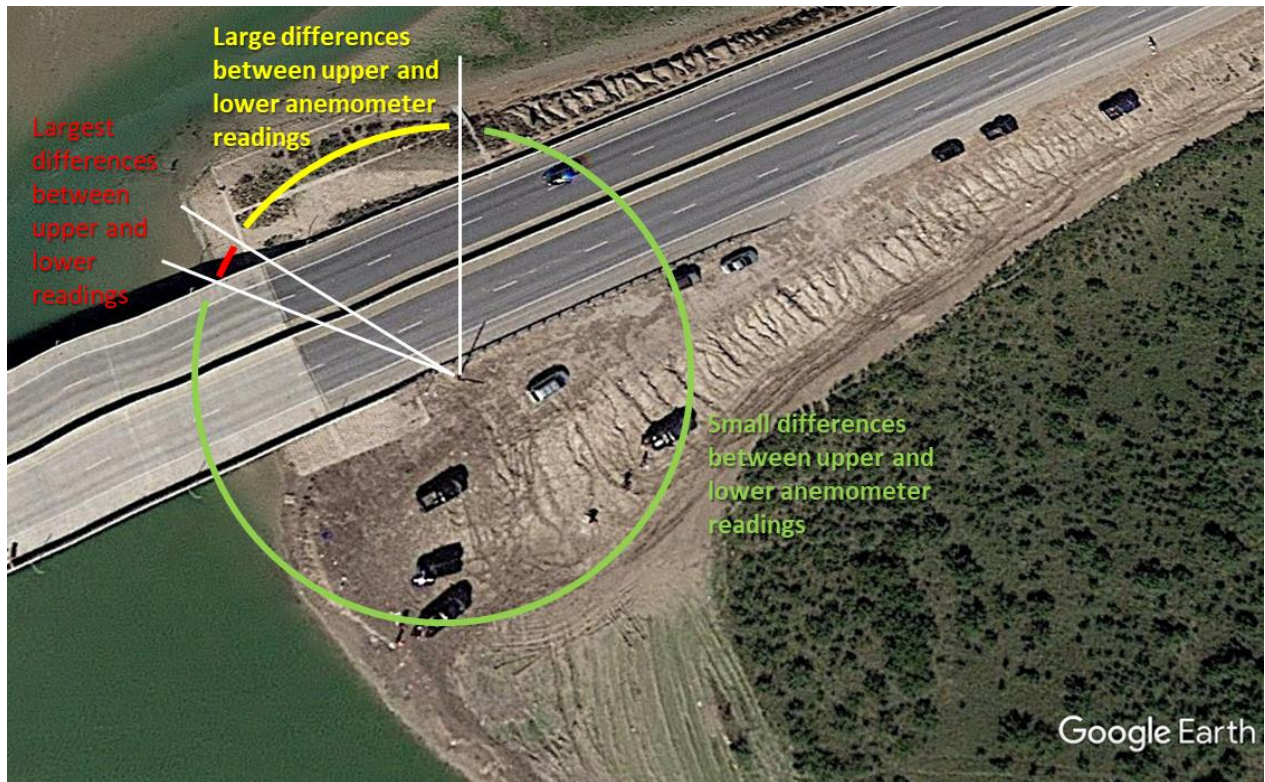
Figure 96. Schematic of Wind Directions That Result in Largest Vertical Differences in Wind Profile Measured by the SH 48 Wind Station.
