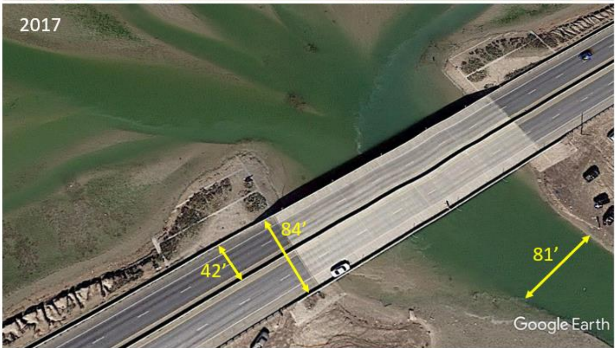
Figure 4. Google Earth Aerial Images (2017) of SH 48, the Carl Gayman Bridge, and Channel after Construction. The lower image provides the inset view of the bridge showing highway width and Bahía Grande Restoration Channel width after the improvements.
