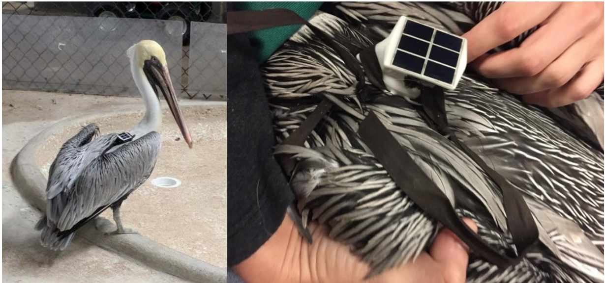
Figure 123. Backpack-Style Transmitter Harness Attached to a Captive Brown Pelican at Dallas Zoo for Practice. The right image shows the Teflon ribbon being tied into a backpack-style harness.
