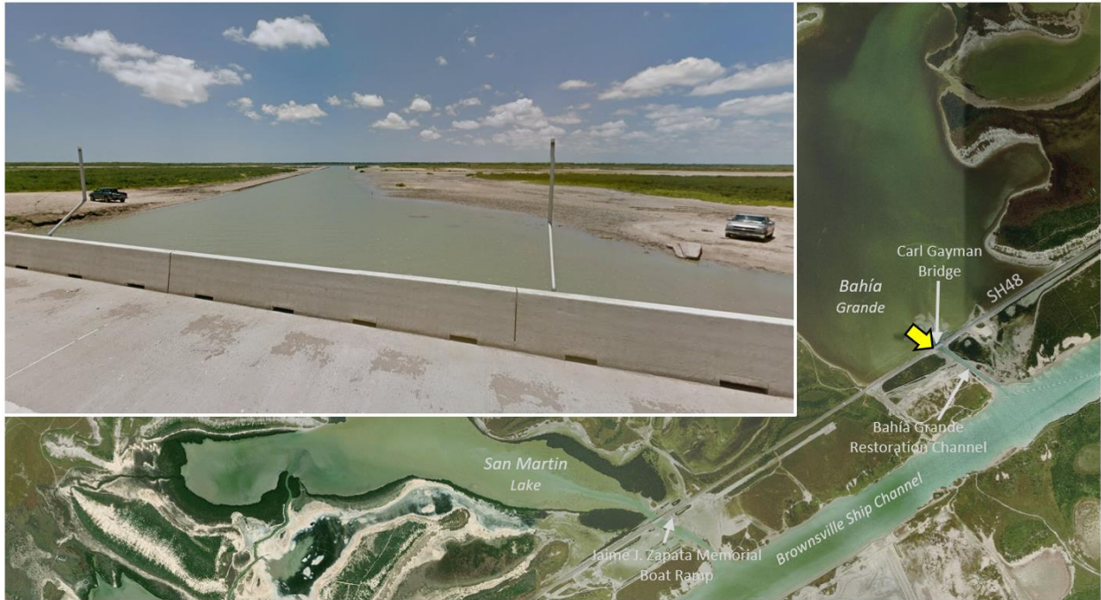
Figure 5. Google Street View of the Carl Gayman Bahía Grande Restoration Channel from Eastbound Lane of SH 48. The Brownsville Ship Channel is located 0.4 miles away at end of the channel. The pelican poles mounted on the 36-inch-high concrete traffic barriers (CTBs) extend 12 feet above the bridge pavement. The yellow arrow on the map indicates approximate photo location and direction (image captured July 2019, view to the southeast).
