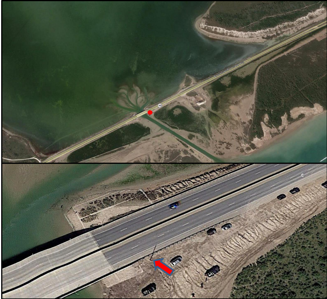
Figure 84. Location of the Wind Station Installed on SH 48. The red dot in the aerial image (top) highlights the wind station with reference to the Bahía Grande, and the Carl Gayman Bridge and channel. The lower aerial imagery shows a finer scale view of the telegraph pole on which the wind station is affixed (marked by the red arrow).
