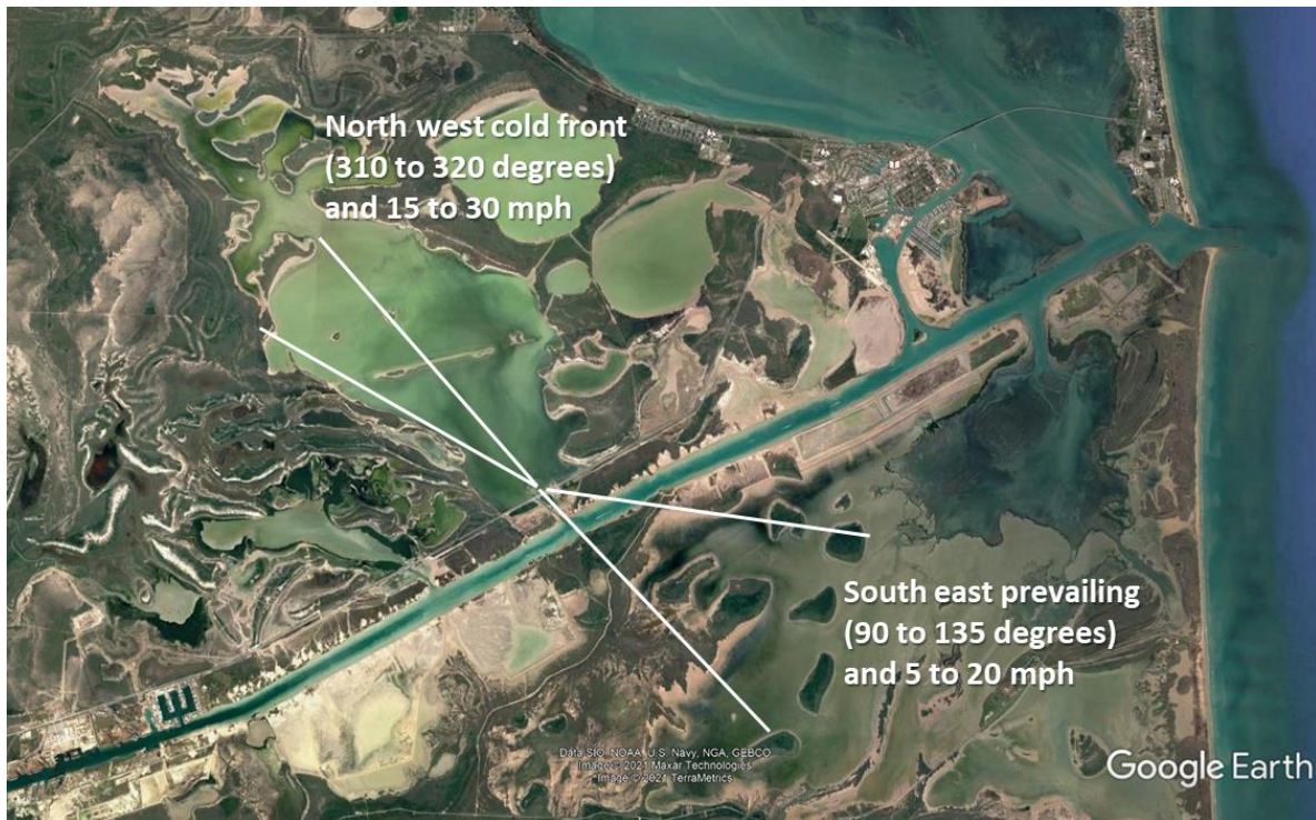
Figure 90. Schematic of Prevailing and Cold Front Winds Measured at the Wind Station on SH 48.
