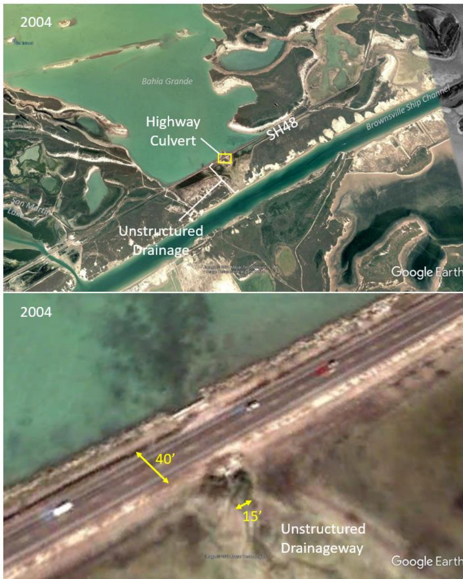
Figure 3. Google Earth Aerial Images (2004) of SH 48, the Carl Gayman Bridge, and Channel prior to Restoration. The lower image provides the inset view of the bridge showing highway and undeveloped drainageway width prior to the Bahía Grande Channel Restoration Project.
