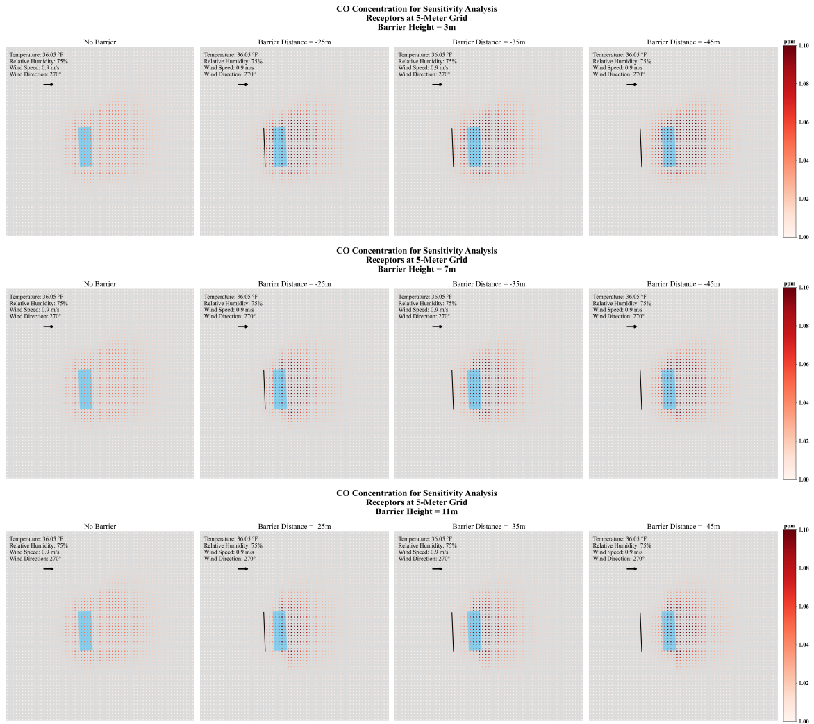
Figure 67 – Predicted CO Concentration by Barrier Height and Distance to Roadway (Barrier Upwind of the Source)
