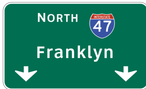
(b) Pull-through sign with down arrows
