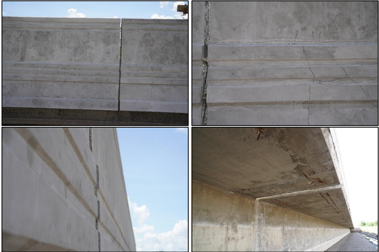
Figure 5.4. Field Side of TxDOT T80SS Barrier with Soundwall after Test No. 440861-4.
