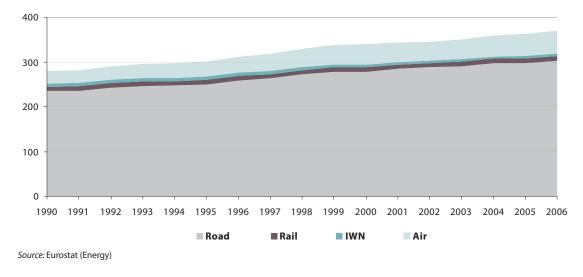
Figure 7.4: Final energy consumption of Road, Rail, IWN & Air, EU-27, 1990 to 2006 (million TOE)
