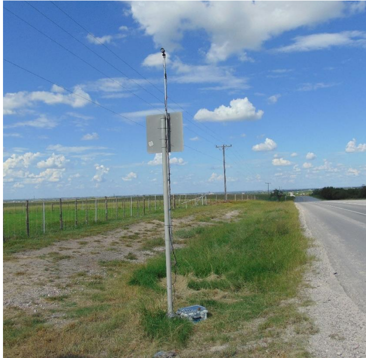
Figure 7. TTI Portable Video Data Collection Equipment.
