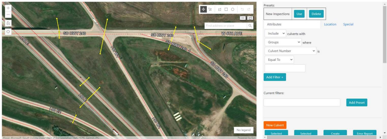
Figure 4. Illustration. SDDOT’s culvert inventory system contains attribute and condition data on over 30,000 culverts along the State highway system. This screenshot from May 2020 shows culvert locations in relation to the highway system.
