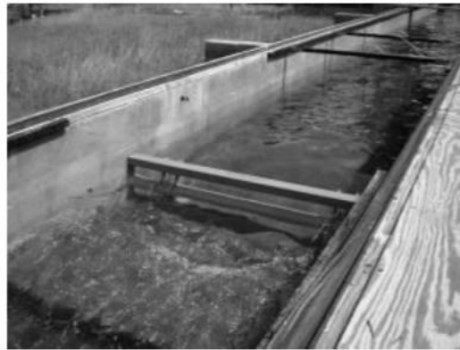
Figure 2.7. Experimental Setup for Bridge Rail in Rectangular Channel.
