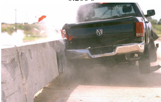
Figure D.2. Sequential Photographs for Test No. 469760-06-2 (Rear View).
