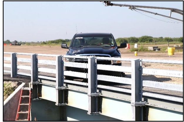
Figure 4.14. TBTA Bridge Rail/Test Vehicle Geometrics.
