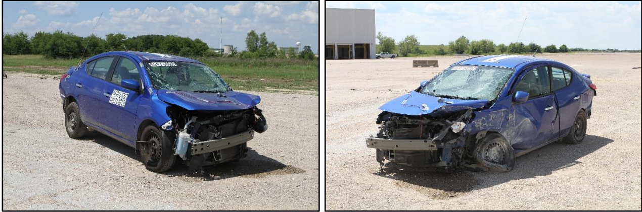
Figure 9.4. Test Vehicle after Test No. 469760-06-1.
