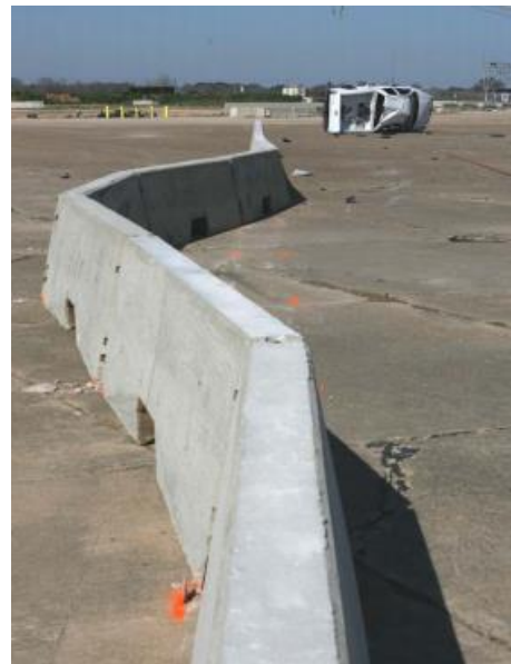
(c) Test Article after Impact
