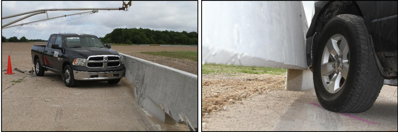
Figure 10.1. TxDOT LSMB/Test Vehicle Geometrics for Test No. 469760-06-2.
