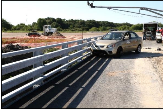
Figure 4.9. TBTA Bridge Rail/Test Vehicle Geometrics.
