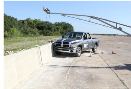
Figure 4.3. Single-Slope Barrier System with and without Test Vehicle before Testing.
