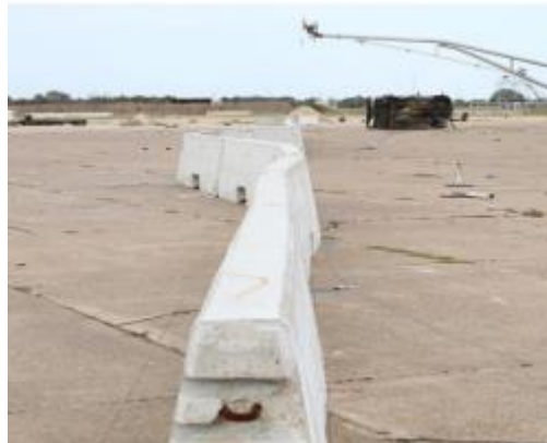
(c) Test Article after Impact
