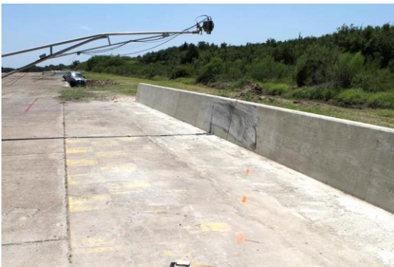
Figure 4.4. Single-Slope Barrier System after Testing.
