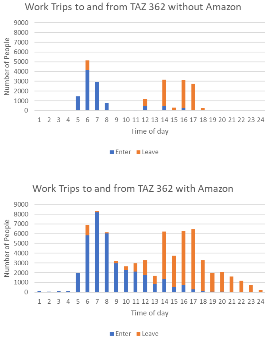
Figure 27. The new HQ is predicted to increase total trips from 5,000 to 8,000 in the morning peak and from 3,000 to 8,000 in the afternoon peak. Late night trips would also expand.
